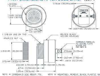
NOTE A: TERMINALS-032 BRASS TIN PLATED, TAPPED FOR #6-32 SCREW. TVD #6-32 NICKEL PLATED BRASS SCREWS INCLUDED WILL ACCEPT 1/4\* OUICK COINNECT. NOTE B: MOUNTING- REMOVE BLACK PLASTIC NUT
