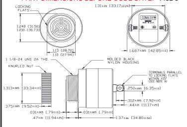
NOTE A: TERMINALS-.032 BRASS TIN PLATED, TAPPED FOR #6-32 SCREW. TWO #6-32 NICKEL PLATED BRASS SCREWS INCLUDED. WILL ACCEPT 1/4\* QUICK CONNECT. NOTE B: MOUNTING- REMOVE BLACK PLASTIC NUT AND INSERT THREADED FRONT THROUGH 1.25' HOLE PUNCHED IN PANEL, IF ORIENTATION IS NEEDED, NOTE LOCKING FLATS ON DRAWING. SCREW NUT BACK ON. DO NOT OVERTIGHTEN.
